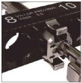
Insert the neutral drill guide into the locking/neutral guide until it securely snaps into place.
