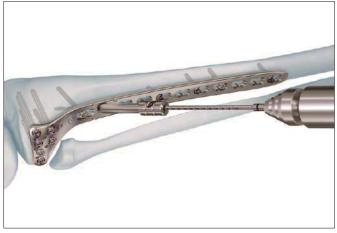
Insert the appropriate length variable angle locking screw.
