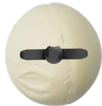
Figure 10. The frontal area of the Hansson Twin Hook is 210 mm 2 .
