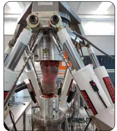
Wrist mounted in Hexapod robot
