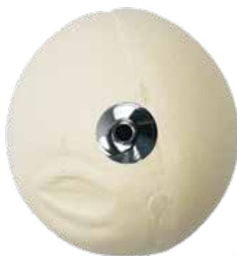
Figure 7. The frontal area of a compression hip screw is 126.0 mm 2 .
