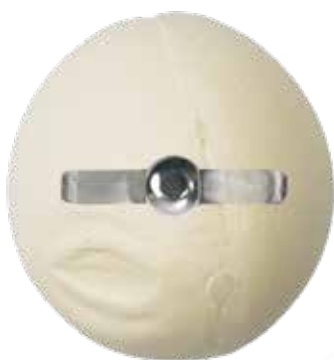
Figure 6. The frontal area of the Hansson Twin Hook is 164.4 mm 2 .
