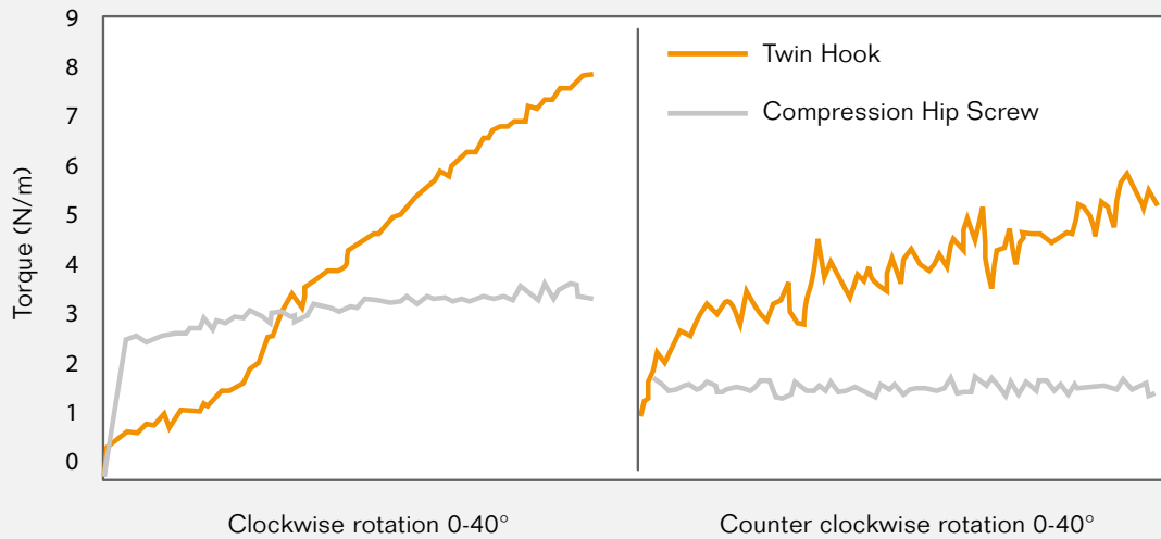
Figure 4. Torque deformation graph showing a comparison of the torsional loading of a Hansson Twin Hook and a compression hip screw during 40° clockwise and 40° counter-clockwise rotation (Ref. 2).
