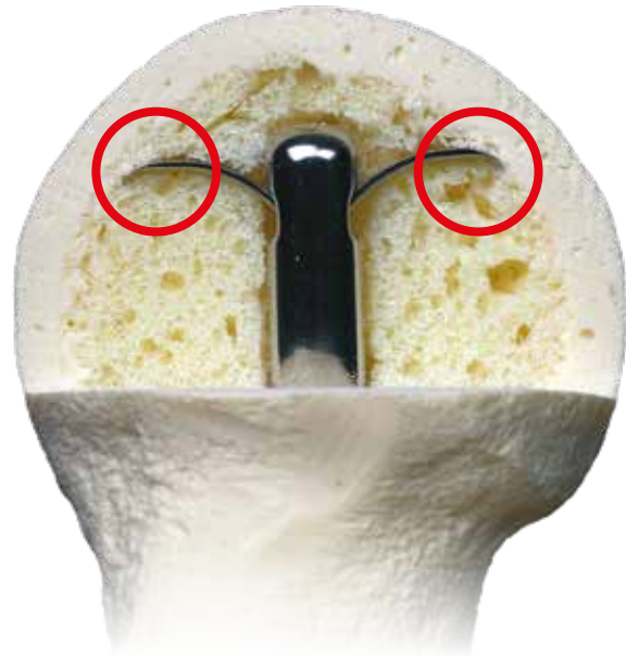
Figure 1. The hooks will be in contact with both cancellous and subchondral bone in the femoral head.
