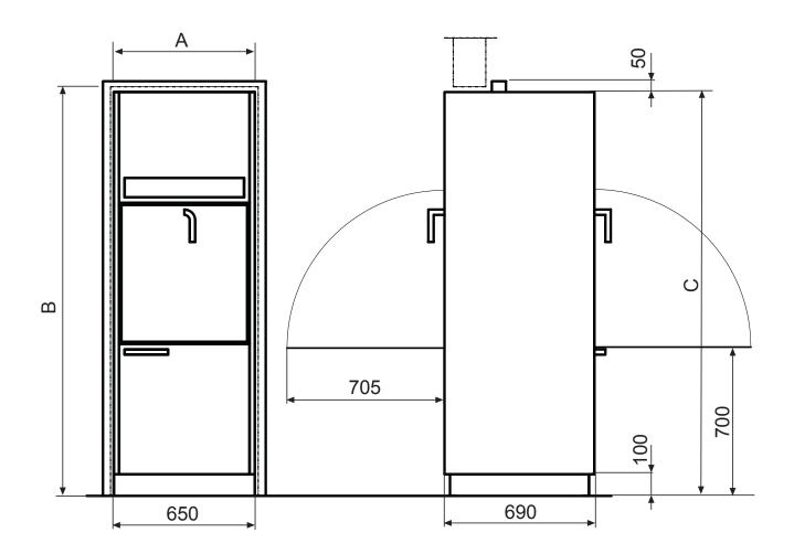
The figure shows trim panels (option) for double door (pass-through) models recessed into a barrier wall. The trim panels cover the gap between the wall and the machine.
