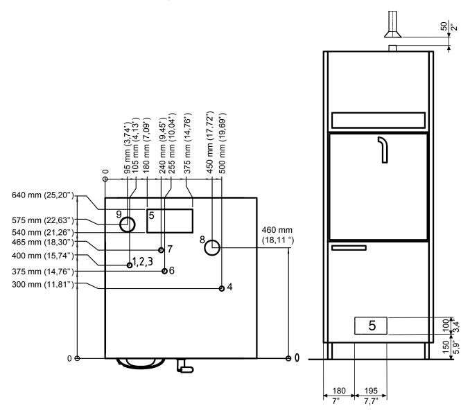
1 Distilled/deionized water 160 mm (6.3") above the floor.
