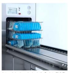
Automatic loader and unloader for Baskets (GL64B).
