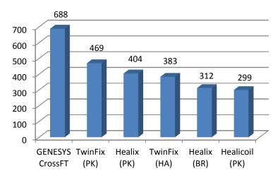
**Figure 1:** Cortical loads-to-failure (*N*) in porcine bone for 5.5mm non-metallic anchors in study.<sup>1</sup>
